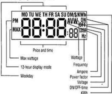
The PM 230 electricity meter is a monitoring and testing instrument with which it is possible to determine the power consumption of a connected appliance and the cost of the electricity consumed.
